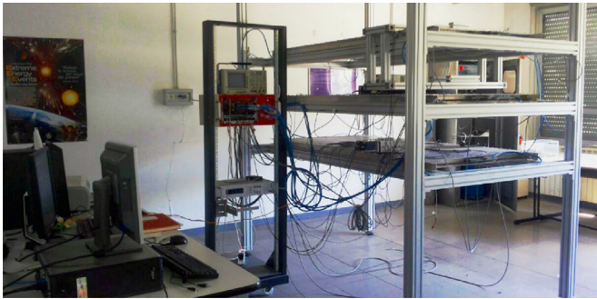
Fig. 2. Picture of the EEE station FRAS-02, located in the high school ITT Enrico Fermi , Frascati (close to Rome). All the basic components of the detectors and the associated data acquisition system are shown: the MRPCs, the VME crate, the low- and high-voltage supply systems, the computer controlling the DAQ and the gas cabinet in the background.
