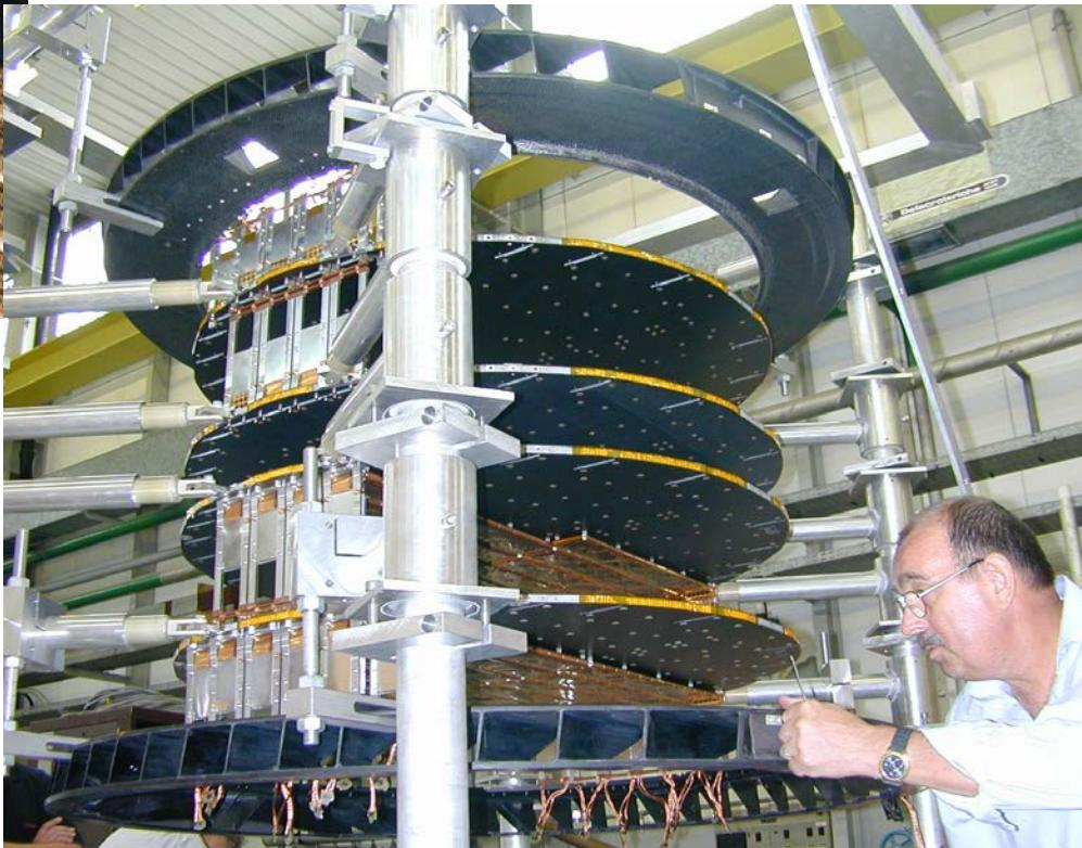
Lightweight carbon fiber shell to hold the planes
