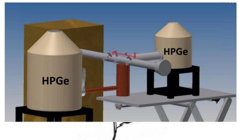
Solution: we use a very well known resonance emitting  $\gamma$  rays in the desired energy range to determine the efficiency
