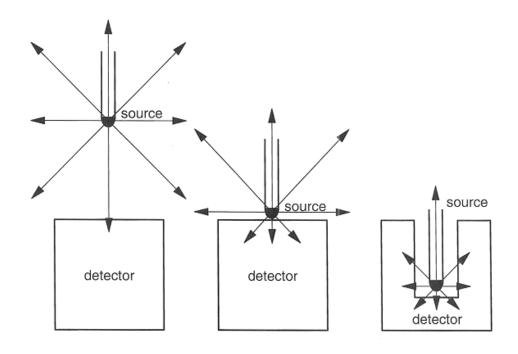
$\epsilon = \frac{\text{number of pulses recorded}}{\text{number of radiation quanta emitted by the source}}$
