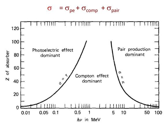
✓ The lines show the values of Z and hv for which the two neighboring effects are just equal
