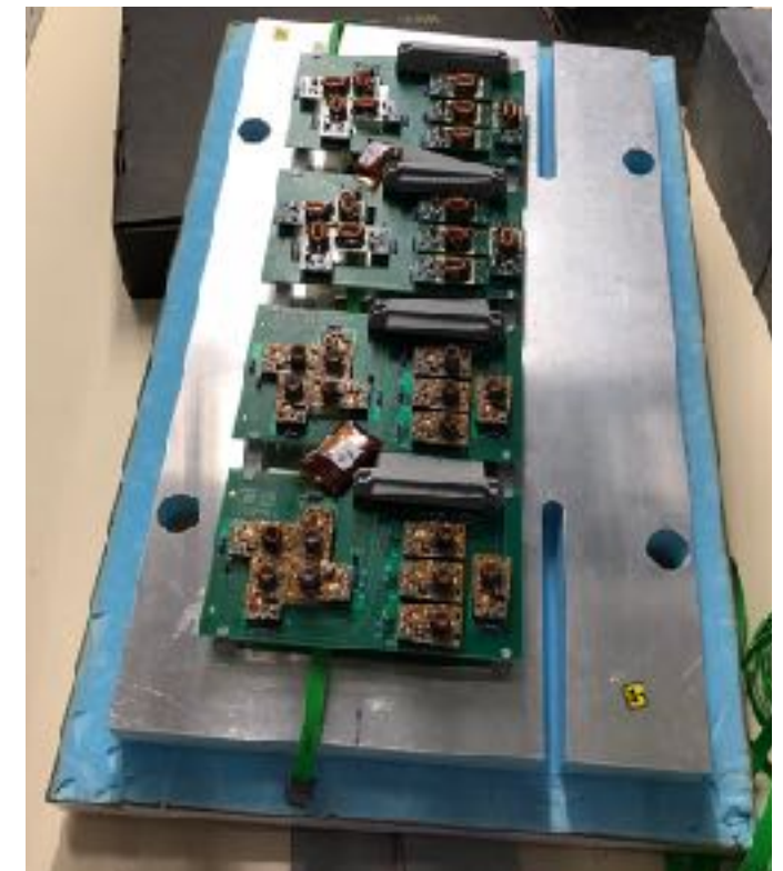
32 modules inside the cold box
