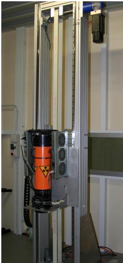
X-rays source 200 kV @ 4.5 mA (for CT scan) 60-90 kV @ 10 mA (for radiography)
