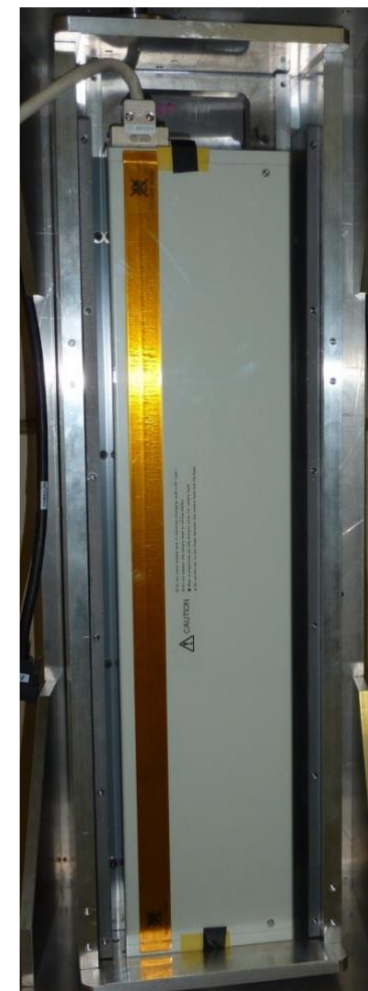
scintillator: GOS (gadolinium-based)
