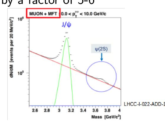
improving low-mass dimuon measurement by reducing the combinatorial background from the semi-muonic decays from kaons and pions and by improving the mass resolution, thanks to the precise measurement of the opening angle of muon pairs
